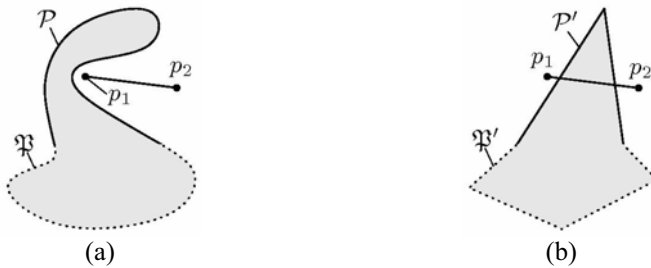
Fig. 5. Case of inconsistency with areal features: (a) original polygon of a subdivision and (b) inconsistent simplified polygon.
