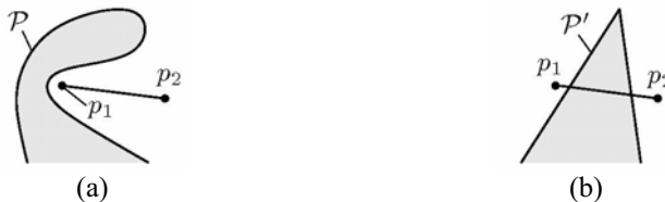
Fig. 2. A case where point feature consistency fails in handling linear features: (a) the original polyline \mathcal{P} and the line segment p_1p_2 , and (b) the simplified polyline \mathcal{P}' that preserves the sidedness of p_1 and p_2 , but intersects p_1p_2 .
